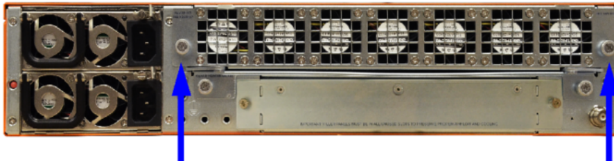
Figure 6 Fan Tray Screw Location on GigaVUE-HC2 Rear
